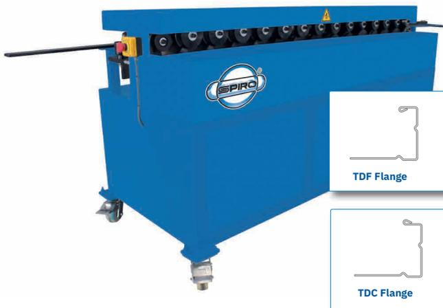
This 14 station Rollforming Machine makes a rigid TDC or TDF flange from hand fed blanks using material from the duct wall.
